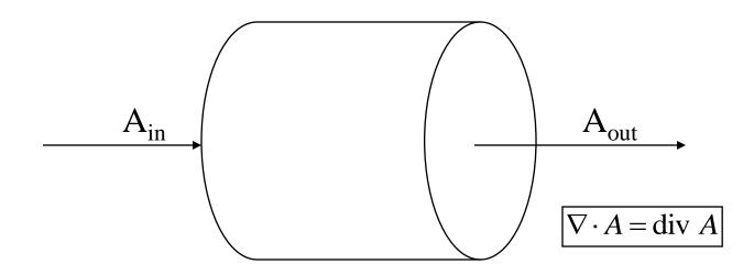
The tubular element is "divergent" in the direction of flow.
